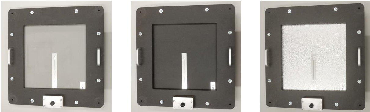
Figure 3.6: Photographs showing from the left the UHPC sample without insulation, the MDF sample with inside insulation and the UHPC sample with outside insulation
