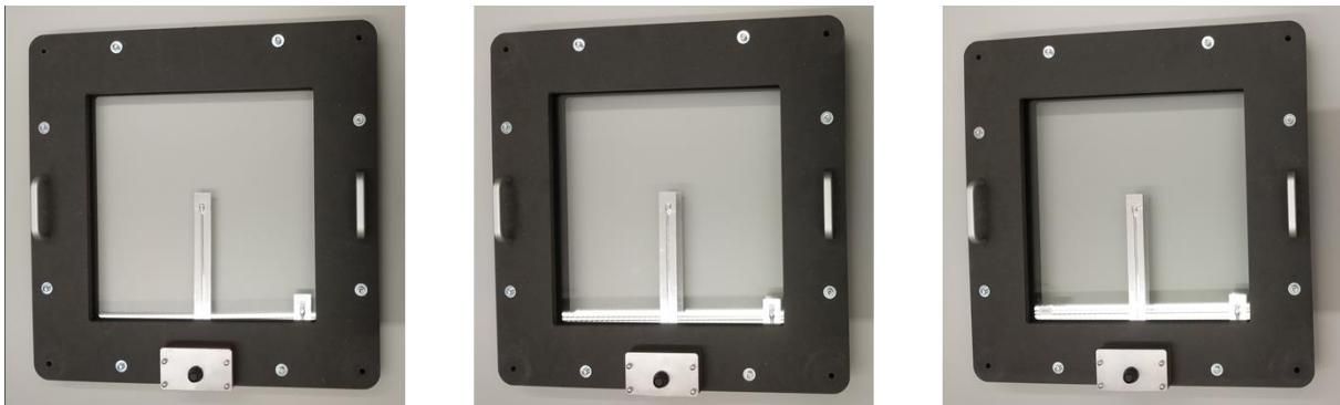
Figure 3.7: Photographs showing from the left the glass sample with single glazing, the glass sample with double glazing and air between the glazing layers and the glass sample with double glazing and argon between the glazing layers
